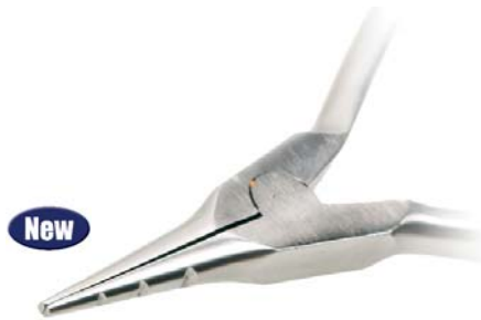
Bow Opening Plier For opening bows or stretching bows and links. Reverse action pliers open when the handles are squeezed. Has ridges to keep the bow in place. Stainless Steel construction. Measures 5 1/2" long overall T-956
